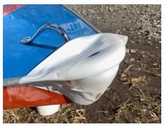
with 80 grit to increase the adhesion potential of the silicone. If you do sand your boat, be sure to wipe all sanding residue off before applying silicone.
