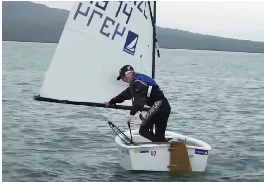
Boom and tiller are facing the same direction while getting out of irons. Which direction will the bow point towards – port or starboard?
